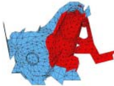
Fifty percent cavity fill of a front-drive transmission case
